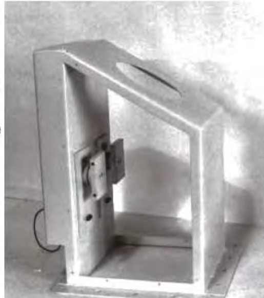
Photo showing the plates attached to the load cells.
