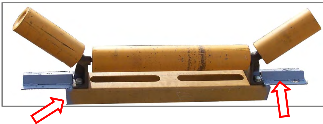
Idler frame is trimmed back and angles are attached to use our V-Block.
