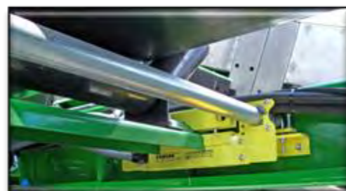
Installed Load Cell Assemblies
