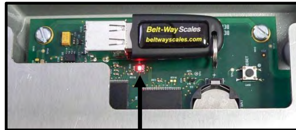
USB Flash Drive Installed on Integrator Board
