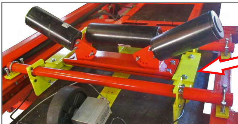
Scale on portable machine using Z brackets
