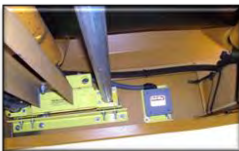
Installed Load Cell Assemblies
