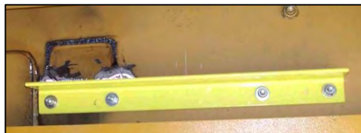
Recessed Mounting Bracket mounted to conveyor frame
